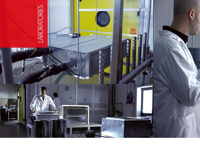
The test chamber has been designed and manufactured with very high quality components, ensuring deviations of  $\pm$  0.2 °C on dry bulb temperature and deviations of  $\pm$  2% on relative humidity.
