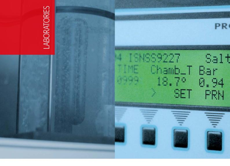
The chamber for salt spray, humidity and cyclic corrosion tests is dedicated to check the corrosion resistance of metallic materials in compliance with the required testing methods indicated by the UNI EN ISO 9227 e EN IEC 60068-2-52 regulations. The test consists of a saline solution nebulized inside the chamber (the bottom is filled with water) obtaining a dense corrosive fog thanks to the use of compressed air saturated with water and from which any oily residues have been eliminated.
