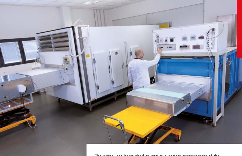
The tunnel has been sized to ensure a correct measurement of the airflow from 90 m $^3/h$  to 6000 m $^3/h$ .
