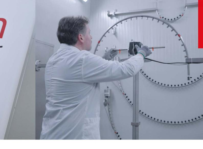
**The IP (Ingress Protection) tests** chamber is used to ensure the protection against rain and water splashes of the electrical enclosures (IPX3 and IPX4 ratings) in accordance with the requirements of EN IEC 60335-1 and EN IEC 60529 regulations.
