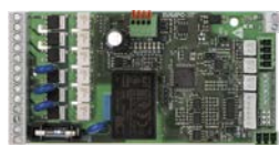
ORT10/ORBT10 OPower card for asynchronous/ brushless motors, for BMS
