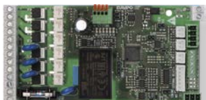
OPower-card for asynchronous motors for BMS (built-in the unit)
